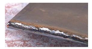
Slag inclusions will normally appear as nonmetallic material along the weld or with the weld metal. Similar to porosity, a maximum size and total length may be indicated.
