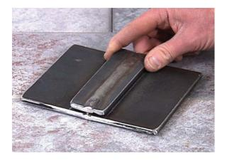
The longitudinal root and face bend are prepared down the weld axis.
