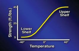
The results of the specimens tested are averaged to obtain a foot pound value at each temperature. The results can be plotted on an energy transition curve. The curves developed for carbon steel show an upper shelf and a lower shelf. The lower shelf indicates that toughness properties are lost in this temperature range. At lower temperatures, steels normally become brittle or lose toughness properties.
