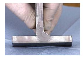
The etchant is normally applied at room temperature using a cotton swab or similar applicator. Etching begins the instant the solution is applied. However, it may be necessary to continue rubbing the surface until there is a clear definition of the weld structure.
