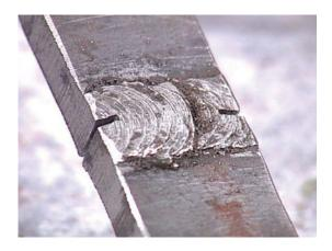
Weld reinforcement is generally not removed so that the entire throat of the weld can be inspected. However, this would not be true with the all-around notch specimen since the notch has removed a portion of the reinforcement.
