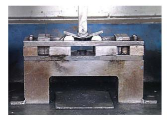
The transverse face bend is positioned in the bend fixture so that the face surface becomes the convex surface of the bend specimen. For a root bend, the root surface becomes convex.
