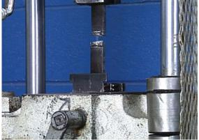
Any suitable means of breaking the specimen is acceptable. However, proper attention to safety must always be considered when conducting the test. The specimens can be pulled in a tension test machine until broken.
