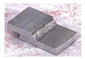
The preparation of pipe specimens consists of welding the prescribed pipe per procedure and then removing the required number of specimens from the required location on the pipe.
