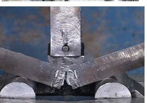
The specimen can also be subjected to a bending load or one end of the specimens could be fixed and the opposite end struck with a hammer to cause the break.
