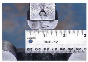
Regardless of the type used, the machine must be set up to provide the required radius on the specimen. The required radius will differ with each code so care must be taken to insure proper set-up.
