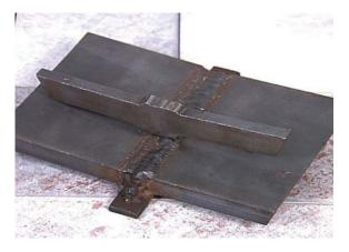
The transverse side bend test is generally used on material greater than three-eighths inch thick.
