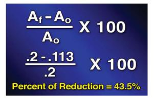
The difference between the original and final area is divided by the original area and then the result is multiplied by 100. A higher percentage indicates greater ductility.
