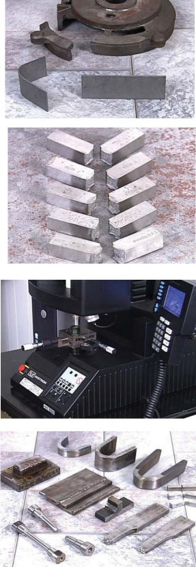
Ductility is the property of a metal which allows it to be drawn or stretched without fracture. A ductile material can be bent. A material which is not ductile is referred to as brittle.
