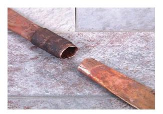
Full sections may be required on thin material or small diameter pipe where it becomes difficult to remove the test specimen.
