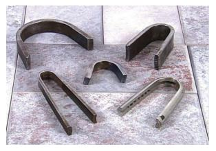
The wrap-around machine is much different. It holds one end of the bend specimen and then forces the other end around a prescribed size die to shape the specimen into a U.
