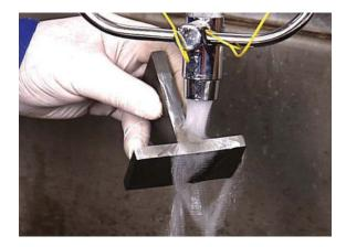
After the surface is completely etched, it is washed in clean water and dried. When handling the specimen, the tester must be careful not to touch the etched surface. The etched surface can be preserved by applying a thin coat of clear lacquer.
