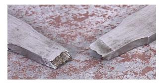
The reduced section tensile is placed in the tension machine and pulled to failure. The strain gage is normally not used to perform these tests.
