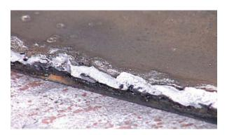
Porosity appears as a round discontinuity on the fractured surface. The discontinuities may have a silver color from oxidation. The maximum size or diameter of porosity and a total size is usually stated by the quality specification.
