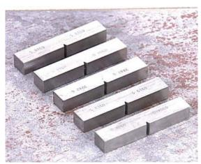
When weld joints require impact tests, a series of specimens are removed transverse to the weld axis. Normally, five, seven or more are required to determine impact properties. The dimensions of the specimens are important to the accuracy of the test. The dimensions are based on the quality specification and the testing procedure.
