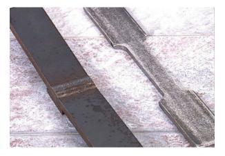
Once the specimens are removed, they are machined to the required dimension. The term reduced section is used since the middle of the specimen is thinner than the ends.
