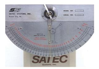
A gage located on the test equipment starts at three hundred foot pounds. The needle will travel clockwise and stop at the top of the pendulum swing.
