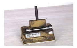
The five-o-five specimen is marked with a centerpunch at two points, two inches apart. This is known as gage length. The original gage length of two inches is recorded for use later to calculate ductility.
