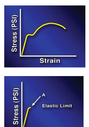
The curve which is plotted is called a stressstrain curve. In the lower part of the curve, the stress is proportional to the strain. Under these loading conditions, the material is an elastic state. This means if the load is removed, the material will return to its original length.
