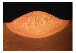
The test outlines or defines the weld structure in relation to the base metal. The etched surface provides a contrast between the weld, heat affected zone and base metal. This form of testing is commonly referred to as metallographic examination.
