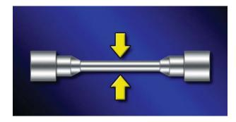
The reduced section of the specimen is normally tapered about .005-inch from the ends to the center. This allows the fracture to occur approximately in the center of the specimen where it is the thinnest.
