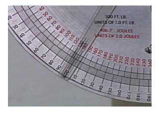
When the pendulum strikes the specimen, it slows down because the specimen absorbs some of the three hundred foot pounds. This prevents the pendulum from making a full swing. At the completion of the swing, the needle will register the amount of absorbed energy.
