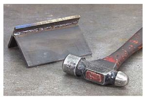
The specimen can be bent or broken using a hammer; or a press could be used to apply a bending load.
