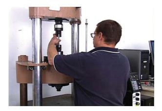
The specimen is secured in the jaws of the tension machine. A strain gage is attached to the specimen to detect changes in length when force is applied.
