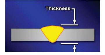
The dimensions of the nick break specimen depend largely on the thickness of the test material and the governing specification.
