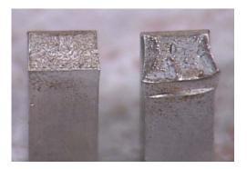
The fractured surface of the impact specimen can also be evaluated at either ductile or brittle. Some standards require that 50% or more of the fractured surface must appear ductile.
