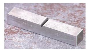
The required numbers of specimens are stamped for identification. Both ends should be stamped so the broken specimens can be matched and evaluated.
