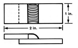
Generally the size of the pipe weld test specimen is at least two inches long and one inch wide. However, the size will vary based on the quality specification. The specimens are prepared, broken and examined.
