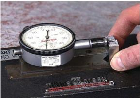
A measure of ductility is also possible. This is the degree of lateral expansion of the fracture surface, sometimes called Mils Lateral Expansion. More expansion on the side adjacent to the notch after testing indicates the material has greater ductility.
