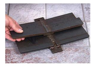
The transverse face and root bend specimens are removed perpendicular to the weld axis. The actual number and location of the specimen will depend on the applicable specification or code.
