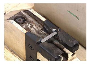
The test specimen is placed at the support fixture against the anvil at the base of the machine. The specimen is supported at both ends and positioned with the notch centered on the opposite side of the pendulum strike.
