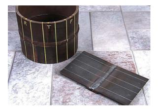
Destructive testing processes are also specified to evaluate the results of welding procedures. Procedure and welders are qualified by destructive tests.
