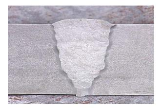
One method of determining metallurgical structures is through etching the welded joint. This method consists of cutting a specimen, polishing the cut surface, applying an etching acid, and visually inspecting the etched surface.
