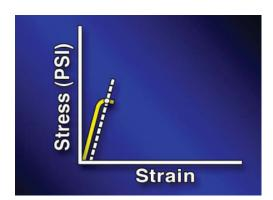
In many cases, the yield point is difficult to determine. Because of this, yield strength is more commonly used to describe the point of yielding, or permanent deformation.
