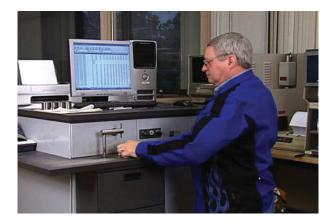
Specialized equipment in laboratory conditions is used to evaluate chemical composition. For example, spectrographic analysis could be used. Chemical composition is important to weldments which require corrosion resistance. Chromium and nickel contents and carbide formations are analyzed to determine the weldment's ability to perform in service.
