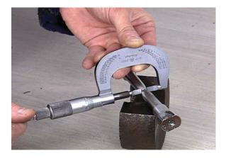
To measure reduction of area, measure the smallest cross section of the broken specimen. Calibrated micrometers or calipers are used to make the measurement.
