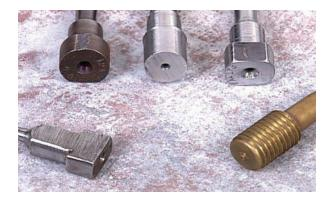
The ends of the specimen are shaped to fit the jaws of the testing equipment in use. Published codes provide requirements regarding preparation of test specimens which must be considered.
