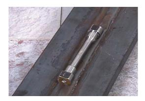
All weld metal specimens are machined from the center portion of a weld test coupon.
