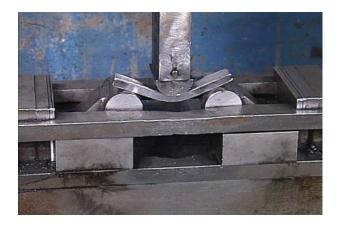
The roller machine works in much the same way. However, the shoulders have rollers attached to minimize resistance during bending.
