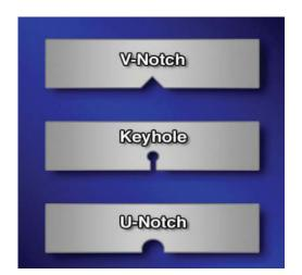
There are three common types of notched specimens used with the Charpy test which include the V-notch, the keyhole notch and the U-notch. The V-notch is the most common. The notch is precisely machined to insure reliability of the results.
