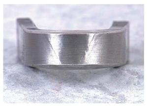
The specimen is bent so that one of the side surfaces becomes the convex surface.
