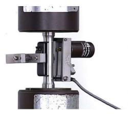
The equipment operator begins the pulling process by allowing the machine to apply pounds of force (load) to the specimen.
