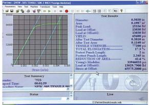
Some tensile equipment is designed with charts to plot the stress in relation to the strain. The gage attached to the specimen detects the elongation which is used by the equipment to plot the strain.
