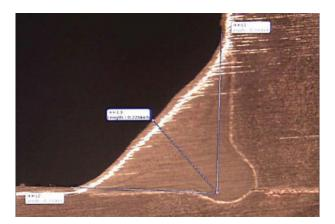
The etched surface is then viewed through a microscope at high magnifications. Usually a picture (micrograph) is produced. The metallurgical structure of the weld metal, fusion zone and heat affected zone are analyzed for characteristics such as grain size, carbon content, and ferrite content.
