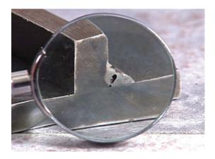
The etched surface is examined to determine weld soundness. Discontinuities such as cracks, porosity, incomplete fusion, slag inclusions and lack of penetration are evaluated.
