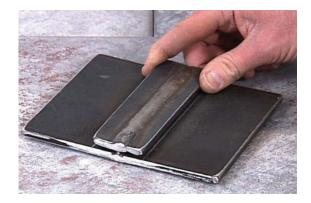
Before bending, the weld reinforcement is removed. Care must be taken to avoid removing material below the surface of the specimen. The grinding or machining should be parallel to the longitudinal axis of the specimen.
