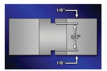
All codes agree that the notch is prepared in the center of the weld. However, the depth of the notch can differ from one code to the next. The notch is prepared by any suitable means. Generally, the notch depth is approximately one-eighth inch. The portion between the two notches is the area of fracture and is normally required to be a minimum of three-quarters inch.
