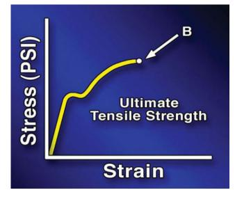
After the material has yielded, the strain gage is usually removed to prevent damage to the gage when the material ruptures.
