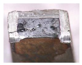
Slag inclusions appear as a non-metallic, glasslike substance on the fractured surfaces. The applicable quality specification will provide dimensions on the amount of acceptable slag inclusions.
