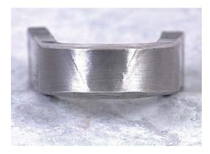
It is used to provide evidence that a welding procedure will produce quality welds with minimum discontinuities. It is also used to determine the welder's ability to deposit sound welds on plate or pipe.
