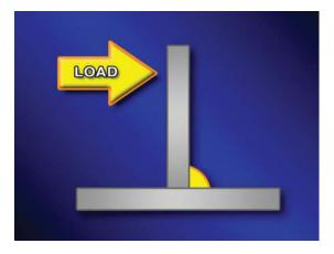
To break the weld, the root must be in tension. Generally, any suitable means of loading the specimen is acceptable although safety must be considered.
