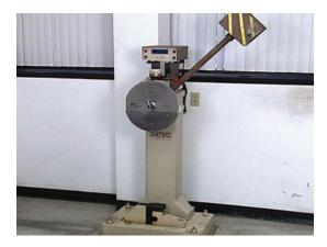
The pendulum is released from a fixed standard height and allowed to swing downward and strike the specimen. As the pendulum falls, it builds up energy.
