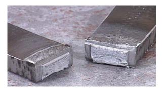
The basic principle of this test is to visually inspect a fractured surface for weld metal soundness. Discontinuities such as porosity, slag entrapment, lack of fusion, or other welding problems are evaluated.
