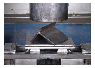
The load is increased or repeated until the specimen breaks. However, if the specimen bends without breaking, it usually passes the test.
