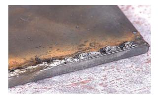
Complete fusion to the root of the joint should be evident. Lack of fusion will normally appear as unmelted base metal with a clear edge.
