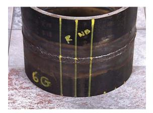
The location from which the specimens are taken is generally the same as for guided bend specimens. However, when both are required from the same test coupon, they are taken side by side, as in the case of certain pipe qualifications.
