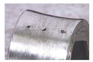
Any discontinuities greater than the allowable code limits are considered unacceptable. For example, the maximum discontinuity size could be one-eighth inch measured in any direction.
