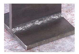
The fillet weld break test is used to qualify procedures, welders and welding operators for producing fillet welds on plate and pipe. It is especially common for the qualification of tack welders.
