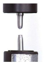
After the ultimate strength is achieved, the actual stress may decrease as the material fails. This is due to the significant reduction of area which occurs in the later stages of the test.
