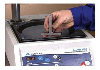
The weld specimens are ground smooth. In the case of carbon steel, the surface can be etched with a solution of one part ammonium persulphate and nine parts water or a solution of diluted hydrochloric acid.
