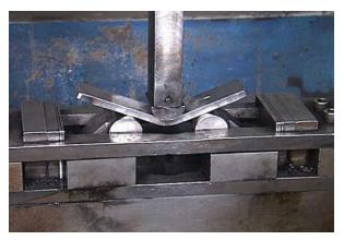
The specimen is placed in the bend fixture with the weld in the center. This insures the weld is in the center of the bend. Activate the plunger and bend the specimen.
