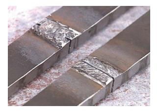
Special attention must be given to the dimensions required. Published welding codes or company standards will dictate the number and type of specimens, if required.
