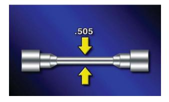
The procedure for testing all weld metal or base metal tensile specimens will be discussed first. It is essential that the applicable specification be reviewed to determine the exact procedure. A .505-inch specimen will be used for illustration.
