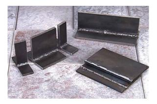
Destructive testing can also be used to spot check the quality of production weldments. This is commonly known as work sampling.
