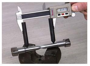
The broken specimen is used to calculate ductility through percent elongation and percent reduction of area.
