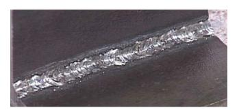
The term weld soundness is commonly used to describe the degree of freedom from discontinuities contained with a weld. Cracks, inclusions, porosity and lack of fusion reduce weld soundness, which may prevent the weld from performing in service. In addition to weld soundness, the mechanical, chemical and metallurgical properties of the welded joint are important to insure reliability of the weldment in service.
