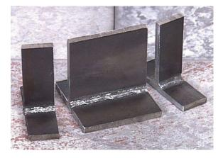
One inch from each end may be removed prior to break testing. This is especially common when macro etch specimens are also required.
