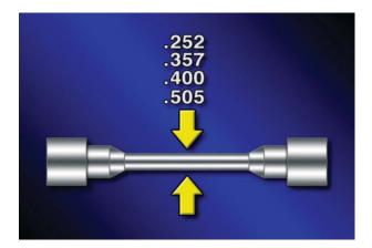
The diameter at the center of the tensile specimen will vary depending on material thickness and code requirements. The finished surface should be smooth enough to prevent premature failure. A rough surface could initiate a fracture in an undesirable location.
