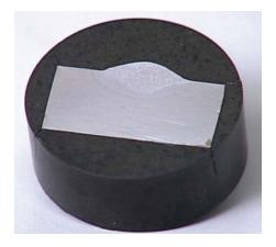
The microspecimen is prepared similar to the macrospecimen. However the surface is carefully ground and polished to a mirror-like finish to remove all scratches.
