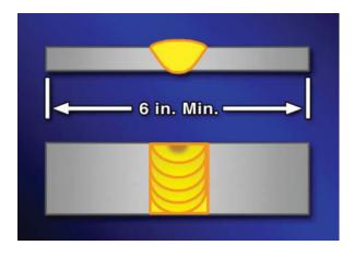
Generally, the length is a minimum of six inches. The width of the specimen is normally no more than four times the test material thickness. The thickness for the transverse face and root bend is equal to the test material thickness and generally does not exceed three-eighths inch.
