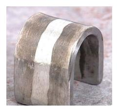
The longitudinal face bend is bent so that the face surface becomes the convex surface of the bent specimen. The root would be tested in a similar manner.
