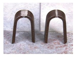
Because it provides a tension and a compression load on a weld specimen, this test is helpful for determining if weld metal and base metal are thoroughly fused.
