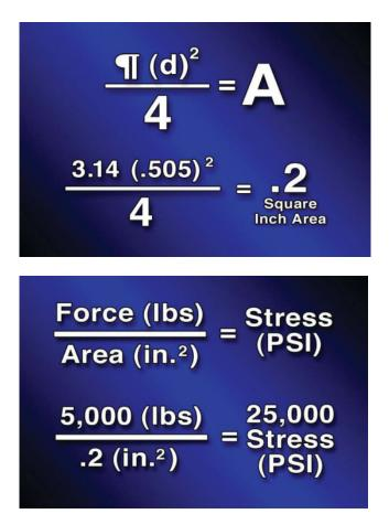
The area of a five-o-five diameter specimen is determined by squaring the diameter and then multiplying by  $\Pi$  or 3.14. This value is divided by four. The answer is .2 square inches.
