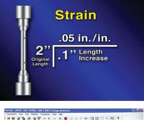
As the force is applied, the specimen begins to stretch or elongate. This is commonly referred to as strain. The units for strain are inch per inch. This is the amount of increase in length per inch of gage length.
