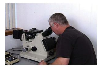
Variations of the process include viewing the etched surface with different degrees of magnification. This form of examination is known as macro or micro examination, depending upon the magnification used.
