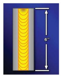
The length is approximately six inches and the width is approximately the width of the weld plus five-eighths inch. The thickness is equal to the plate thickness up to a maximum of three-eighths inch.
