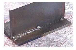
The preparation for the t-joint test consists of depositing the proper size fillet weld according to the welding procedure. Some codes may require a weld restart in the center of the bead.
