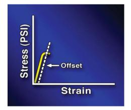
This is described an as offset method since the distance between the lines is a percentage of the original gage length. The point at which the offset line crosses the original curve is the yield strength.
